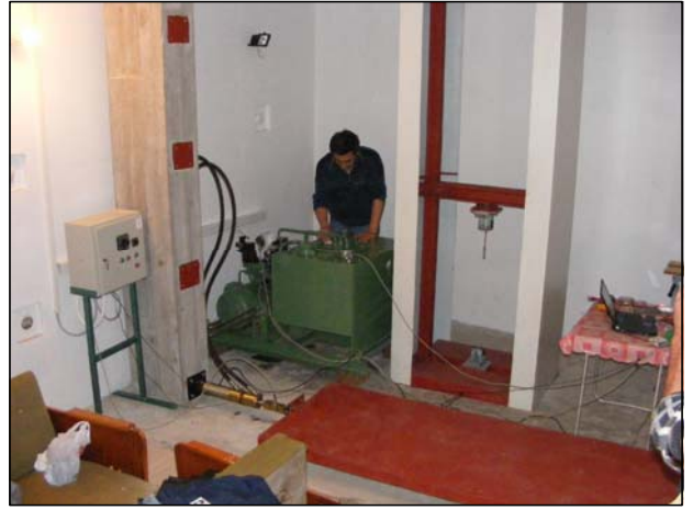
Vibro-platform, actuator frame and column for horizontal load
