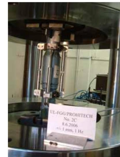
Damper during the testing, 1-5Hz.
