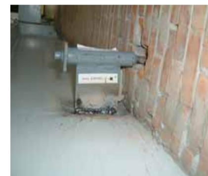
Applied damper model in ratio 1:27 to a wall model on a vybro-platform in Skopje.
