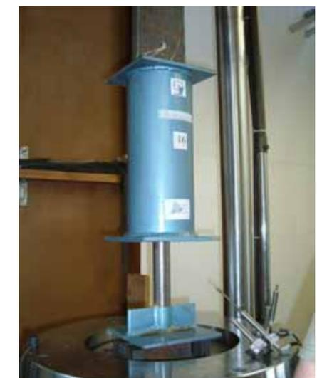
Compensator of displacement during the testing (0.001Hz) in Ljubljana.
