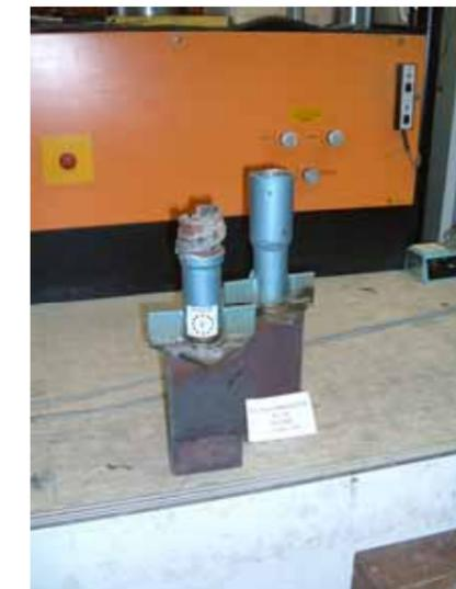
Damper after the break in process of the testing.
