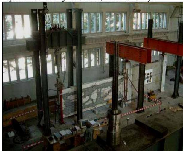
**1. System DC 90 strengthening of EXISTING MASONRY OBJECT in aim of stiffening to horizontal influences (wind and earthquake), acceleration of building procedure, costs decrease and enduring lasting period of the object means**
