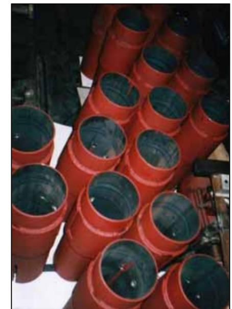
A damper series for RC frame constructions before delivery.
