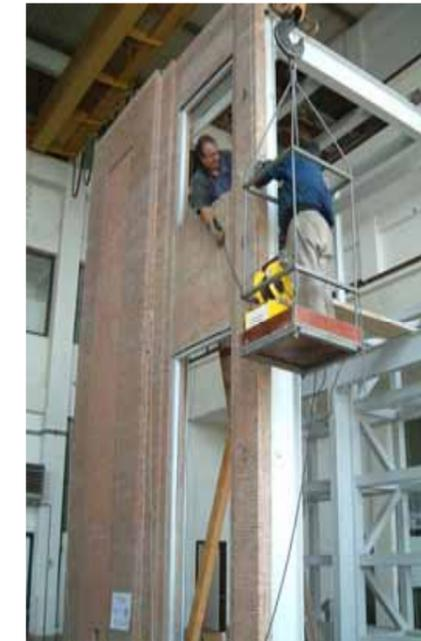
Applying damper model in ratio according to forces 1:27 on a wall model R=1:3.
