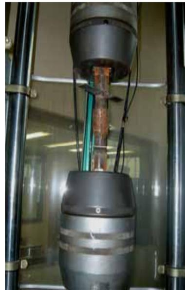
Damper testing to dynamic load in frequent range 1-10Hz in Military-Technical Institute VTI, Zarkovo, Belgrade and damper work-check to low-cycle fatigue in post-elastic field.
