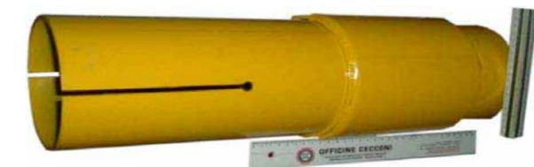
1. Damper for RC frame structures to be built in places of plastic hinge in frame-structure building beams. The diagram of the damper is decided according to reinforcement diameter ( $\emptyset 12 - \emptyset 30$ ).
