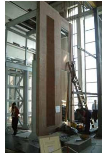
Model of the wall of hydro-generator "Beauharnois" in 1:3 ratio on vybro-platform
