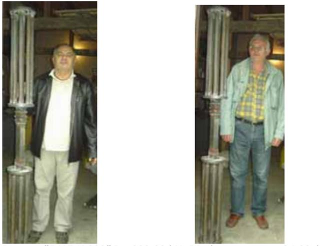
Damper "BAKI K 900" P= 900.00 kN, Displacement = +-24.00 / +24 MM.
