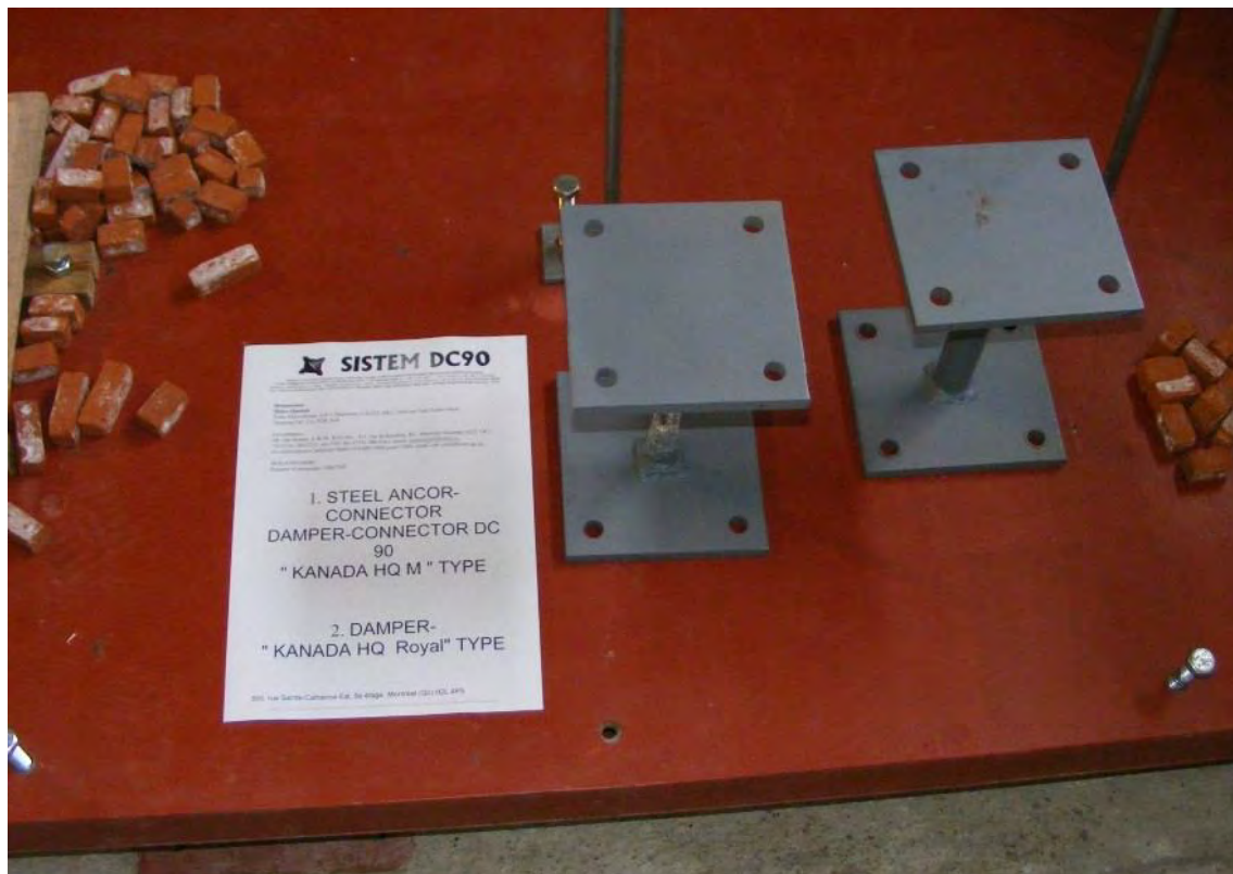
Figure 10. View of Damper type “Canada” (absorber of seismic energy).
