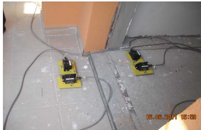
Figure 27 Separation joint- forced vibration test
