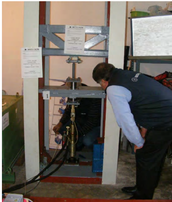
Figure 1. AFS, Servo-controlled Hydraulic System
