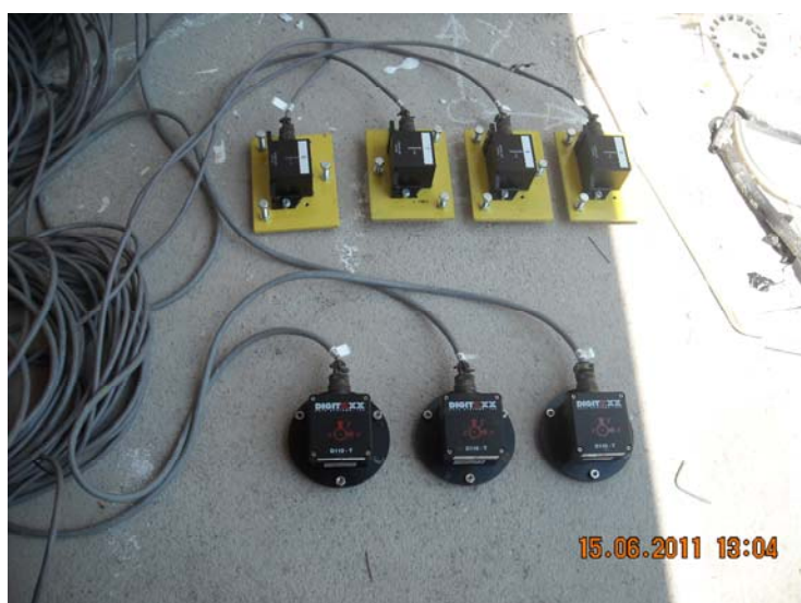
Figure 12. Dynamic calibration test of DIGITEXX accelerometers
