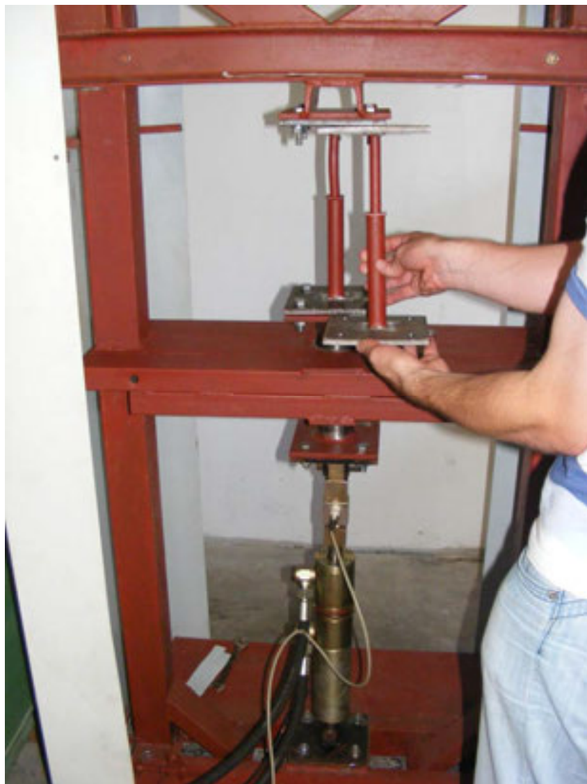
Figure 9. View of Damper type “Canada” (absorber of seismic energy).
