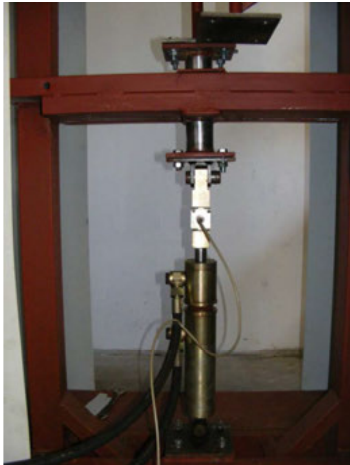
Figure 1. AFS, Servo-controlled Hydraulic System
