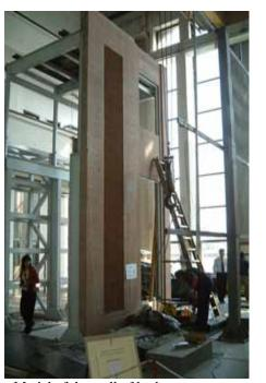
Model of the wall of hydro-generator "Beauharnois" in 1:3 ratio on vybroplatform
