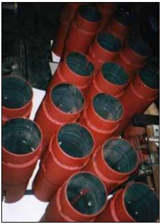
A damper series for RC frame constructions before delivery.
