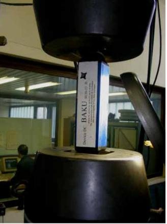
Test of Damper made of stainless steel Cr-Ni assigned for Hydroelectric Power Station in Quebec, Canada
