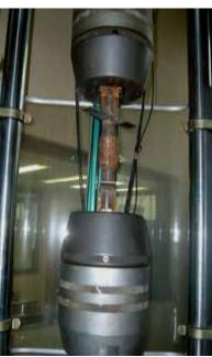
Damper testing to dynamic load in frequent range 1-10Hz in Military-Technical Institute VTI, Zarkovo, Belgrade and damper work-check to lowcycle fatigue in post-elastic field.
