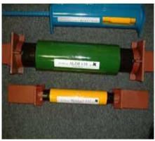
Applied damper model in ratio 1:27 to a wall model on a vybro-platform in Skopje.
